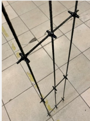
Composite mesh with enlarged plastic connections
