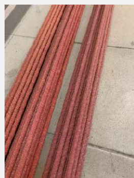
Production of colored composite rebar
